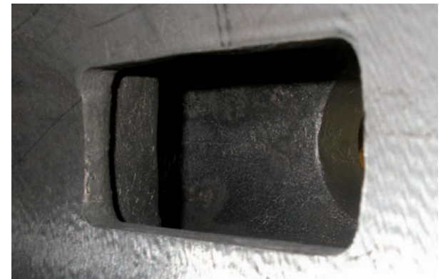
Image 5: Control channel made of CERATEC
