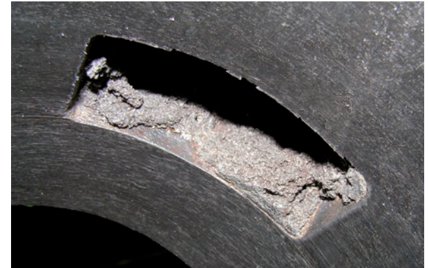
Image 4: Control channel with mineralization (chromite core)
